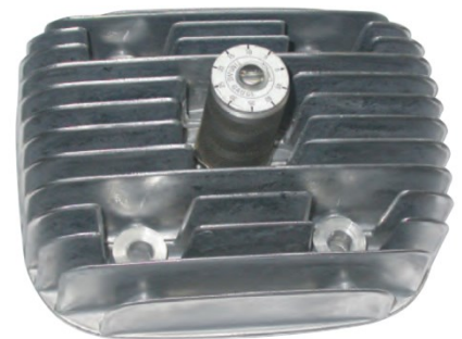
Cylinder head with ignition timing tool
